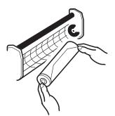
3 Load the instrument with the paper, putting it into the holder.
